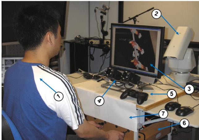
Fig. 7. Experimental setting: (1) participant, (2) remote camera, (3) screen view of video stream, (4) eye tracker, (5) gamepad as joystick control, (6) re-designed foosball game, (7) covers to obscure participant's direct view of the foosball table.
