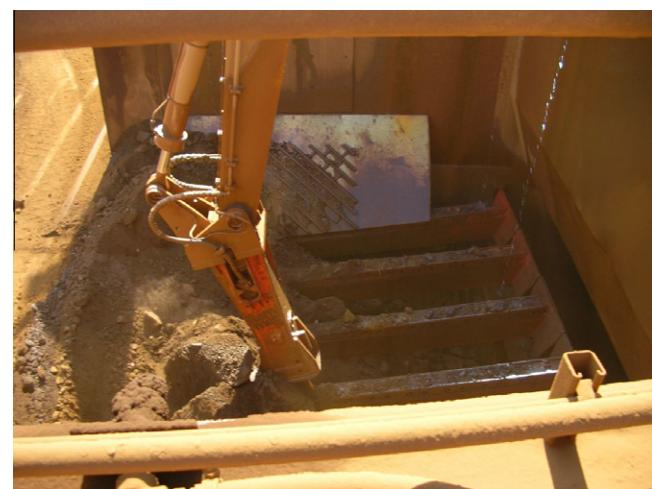
**Fig. 2.** The ROM bin with a grizzly at the bottom.
