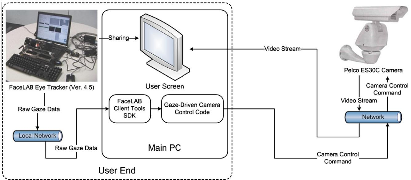
**Fig. 5.** System diagram for the implementation of the gaze-driven camera control prototype.
