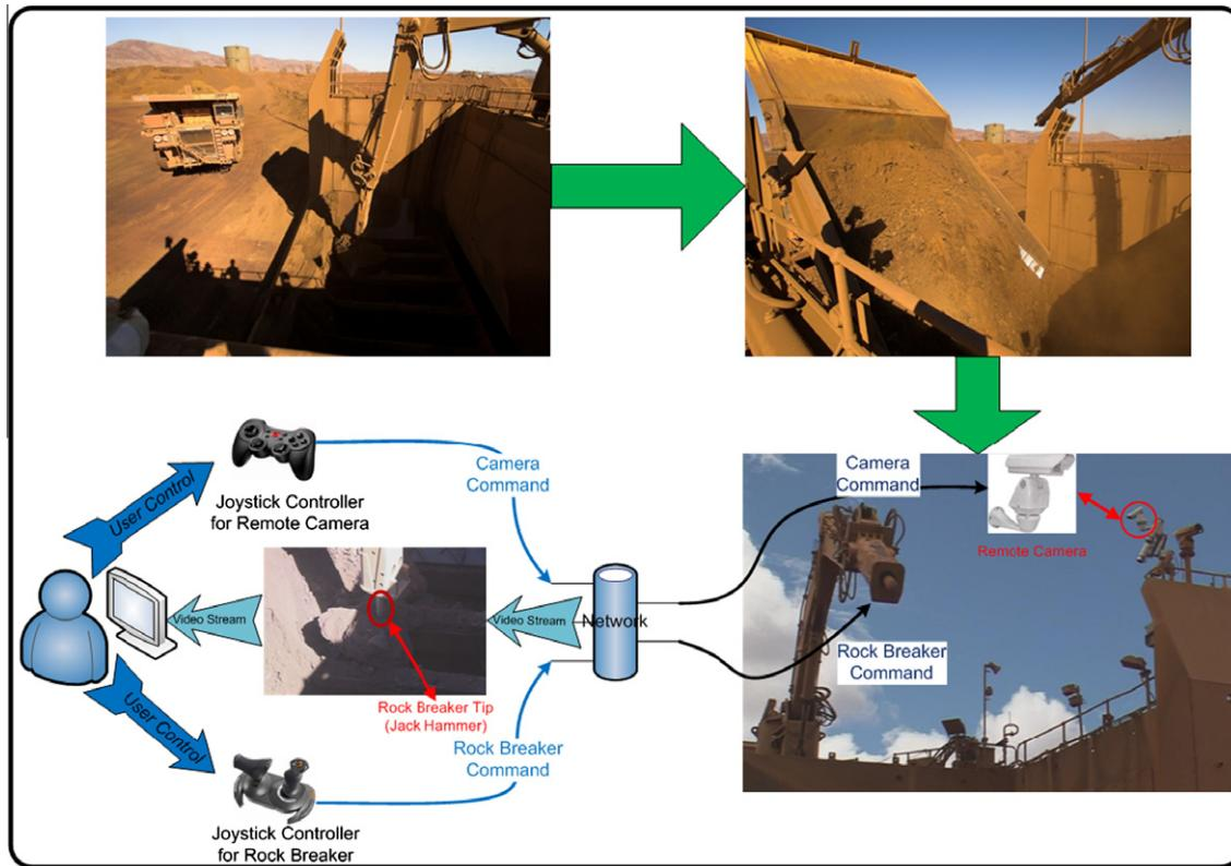
Fig. 3. Remote rock breaking.
