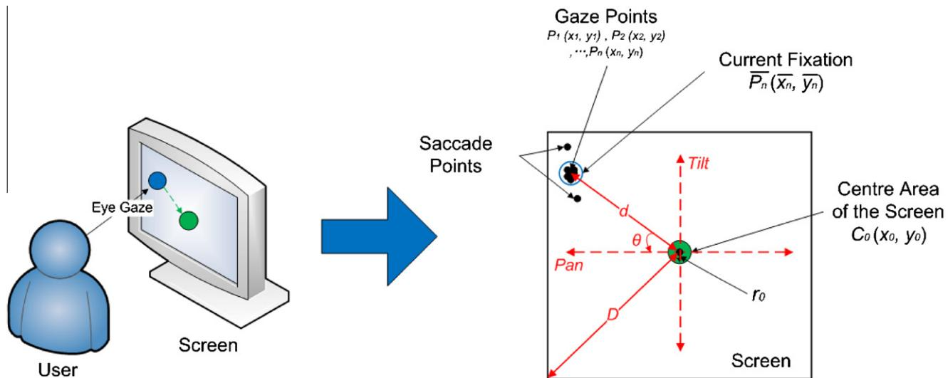
**Fig. 4.** Design of gaze-driven remote camera control.
